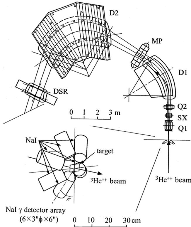
**Fig. 48.** RCNP spectrometer Grand Raiden and the  $\gamma$ -detector array. D1 and D2: dipole magnets. Q1 and Q2: quadrupole magnets. SX: sextupole magnet. DSR: dipole magnet for spin rotation. MP: multipole field magnet. NaI detector array is for  $\gamma$  detection in coincidence with CER particles [93].
